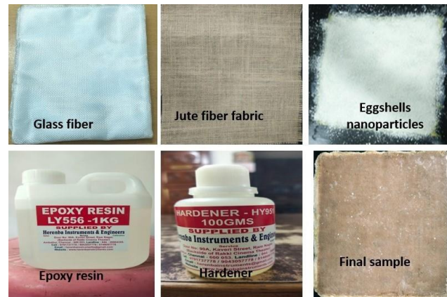
Fig. 1. Materials used for fabrication of hybrid composite
