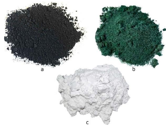
Fig. 3. Synthesis stages of the sample: a – titanium slag; b – titanium slag after reaction with NaOH; c – calcined product after hydrolysis
