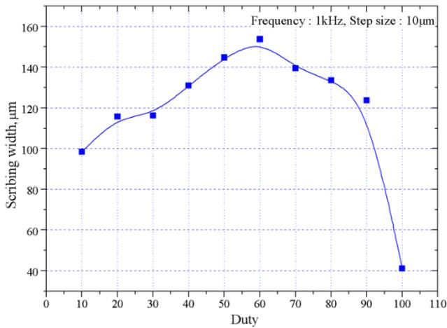
**Fig. 5.** Change of scribing width after laser beam irradiation
