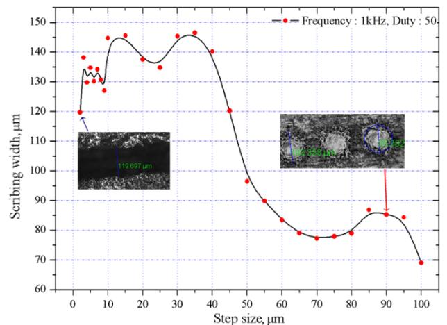
**Fig. 6.** Scribing width according to change of overlap of overlap
