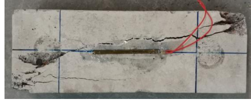
Fig. 4. Uniaxial compression failure mode
