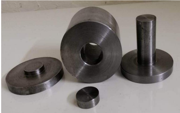
Fig. 1. The mold used for pressing powders [1]
