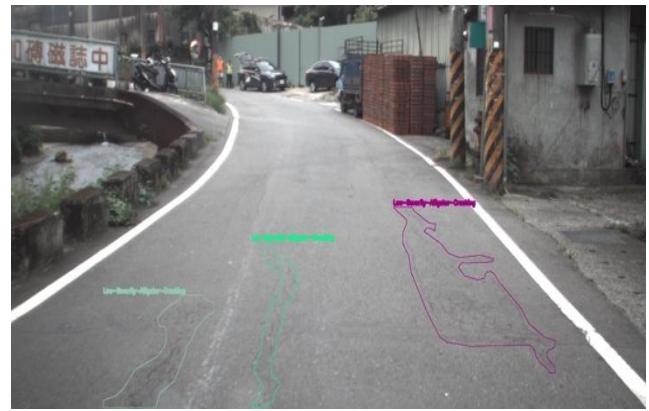
Fig. 1. Pavement distress identification (forward view, YOLO V8)
