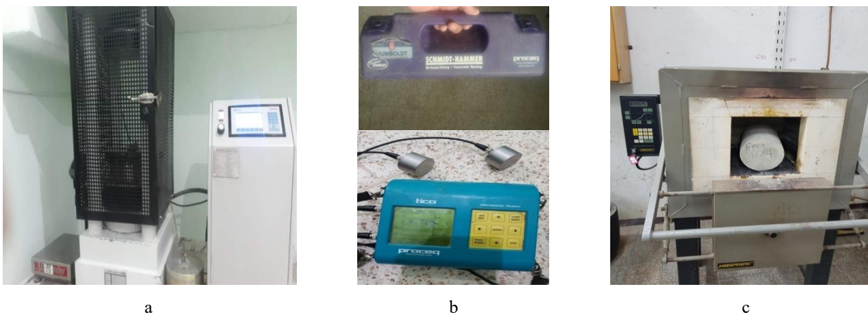
Fig. 1. Test equipment and instrumentation: a–compression testing machine; b–Schmidt hammer and ultrasonic pulse velocity; c–programmable electrical furnace with integrated temperature controller
