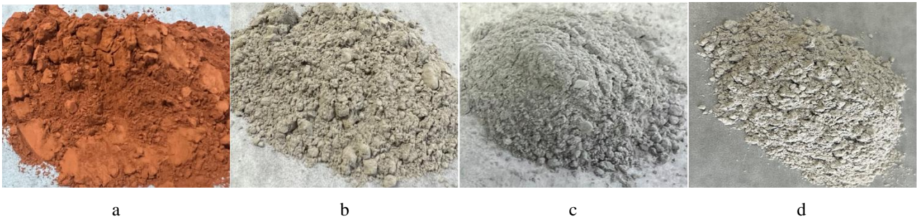
Fig. 1. Morphology of : a – red mud; b – fly ash; c – silica fumes; d – ordinary Portland cement
