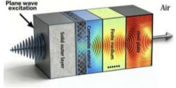
Fig. 2. Theoretical model of the transfer distribution of a composite structure
