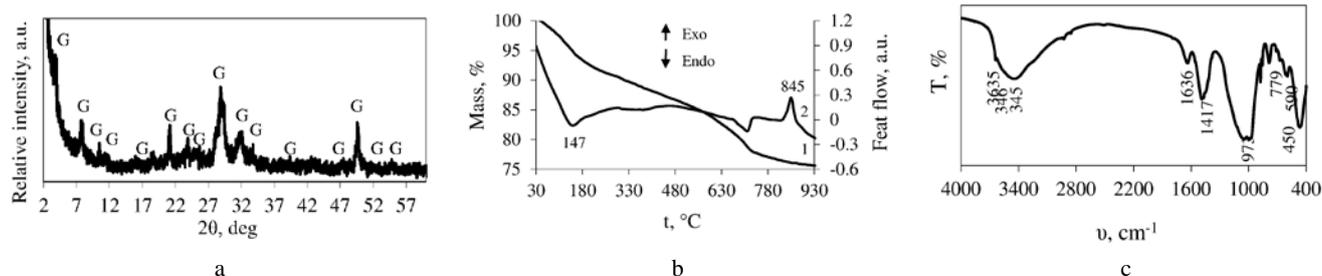
**Fig. 6.** X-ray diffraction pattern (a), DSC – TG curves (b) and FT-IR spectrum (c) of gyrolite substituted with Fe<sup>3+</sup> ions. Indexes: G – gyrolite
