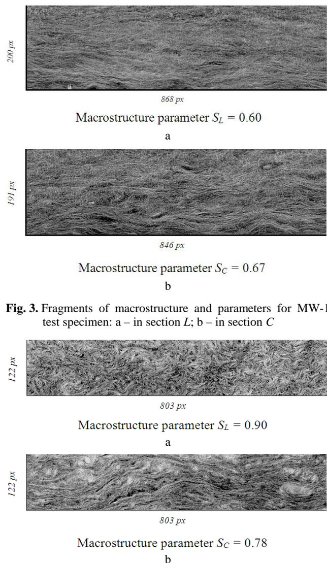
**Fig. 3.** Fragments of macrostructure and parameters for MW-1 test specimen: a – in section  $L$ ; b – in section  $C$
