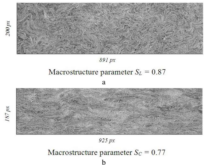
**Fig. 9.** Fragments of macrostructure and parameters for MW-7 test specimen: a – in section *L*; b – in section *C*
