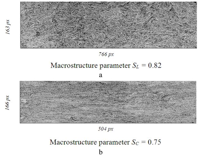
**Fig. 8.** Fragments of macrostructure and parameters for MW-6 test specimen: a – in section *L*; b – in section *C*
