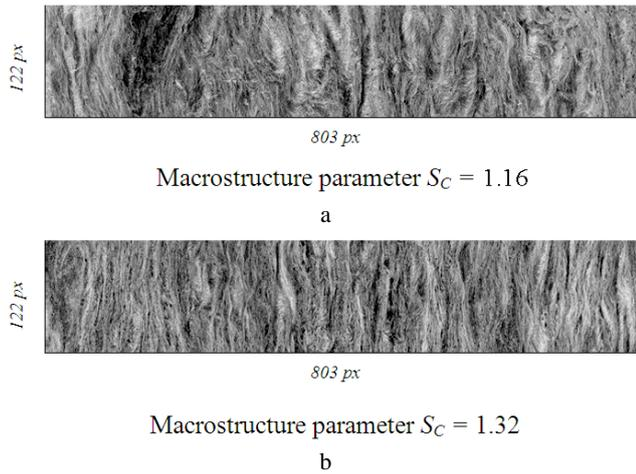
**Fig. 5.** Fragments of macrostructure and parameters for MW-3 test specimen: a – in section *L*; b – in section *C*
