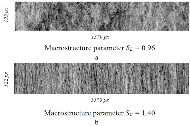
**Fig. 7.** Fragments of macrostructure and parameters for MW-5 test specimen: a – in section *L*; b – in section *C*
