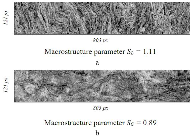
**Fig. 6.** Fragments of macrostructure and parameters for MW-4 test specimen: a – in section *L*; b – in section *C*
