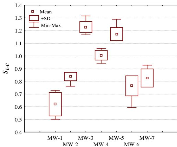
**Fig. 10.** The spread of the average values of the macrostructure parameter  $S_{L-C}$  for all types of test specimens
