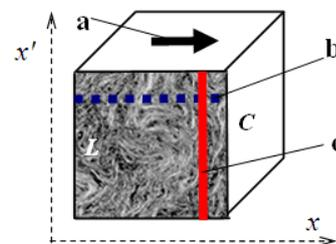
**Fig. 2.** The surface of the test specimen in *L* section with a chaotic structure: a – direction of fibre web movement; b – orientation of fibres in parallel to axis *x*; c – orientation of fibres perpendicularly to axis *x*
