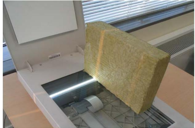
**Fig. 1.** Scanning of surface of test specimen by scanner
